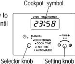
If the oven is switched off on the wall, or there is a loss of power, the clock will stop and you will not be able to use the oven. When you first switch the electricity supply on, the timer display will flash.
